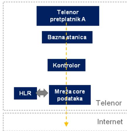
Figure No.1 in Table A8 is related to the traffic of calls within the network. The Figure shows the flow of such traffic, which, on that occasion, employs one MSC/MSS/MGW, one BSC/RNC controller twice, two base stations.
